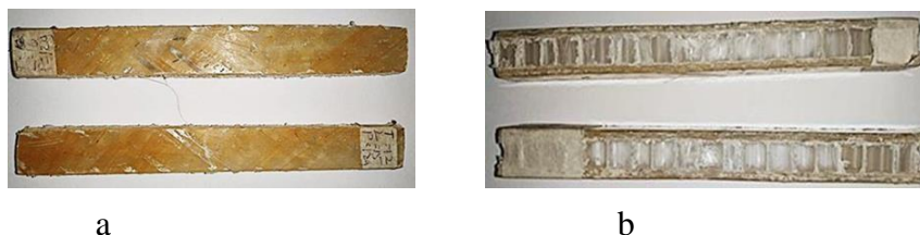
Figure 6 Failure Mode Impact Strength of Sandwich Composite Other Unbroken: a. Delamination age middle, b. Failure in core
