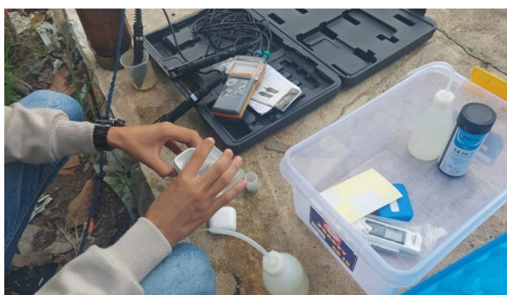
Figure 2 The process of measuring pH, temperature, DO, and TDS using water quality testing.
